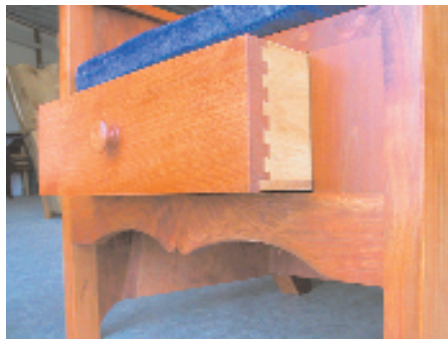
One of Fisher's early lambing chairs, together with a detail of the drawer construction.
